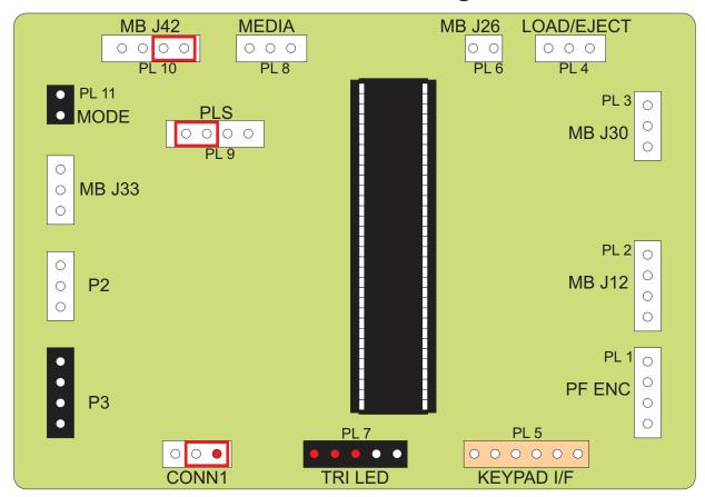
KEYPAD I/F (PL 5) Keypad Interface TRI LED (PL 7) Three way LED PLS (PL 9)
